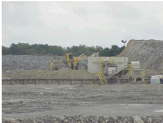
**Figure 4.28:** Mobile crusher and XRF unit (Copyright Halliburton Energy Services).
