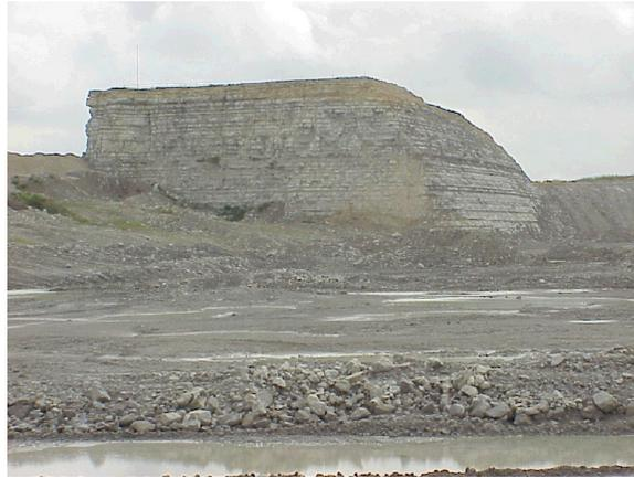
**Figure 4.27:** Limestone quarry formation, showing the 45° ripping technique (Copyright Halliburton Energy Services).
