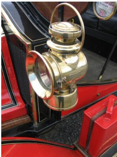
**Figure 4.20:** The carbide lamp on a 1911 Renault.
